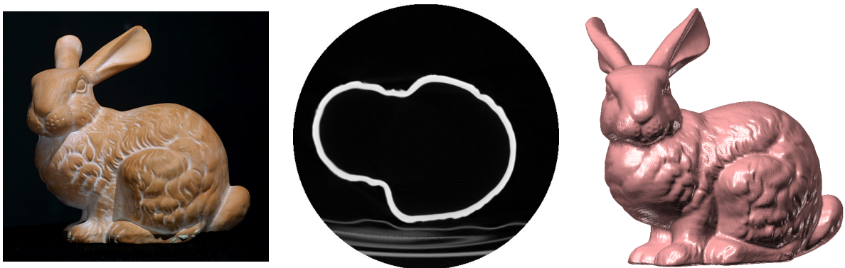
Fig. 1.2. Shape acquisition with an X-ray CT scanner. Left: original 3D object. Middle: a horizontal slice of CT-scanned image. Right: isosurface of CT-scanned image. The left and the center images are courtesy of the Stanford Computer Graphics Laboratory.
