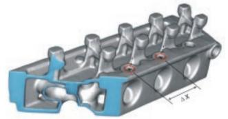
CT-measured automobile cylinder head right: distance measurement of two channels, front left: virtual cut of the CT-measured data
